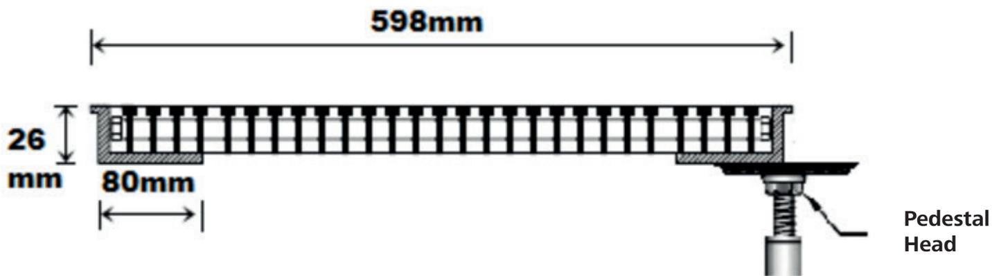
Computer room floor grille fitted with opposed blade damper (OBD)
